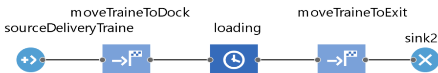
Fig. 2. Discrete-event process of simulating the arrival and departure of covered cars
