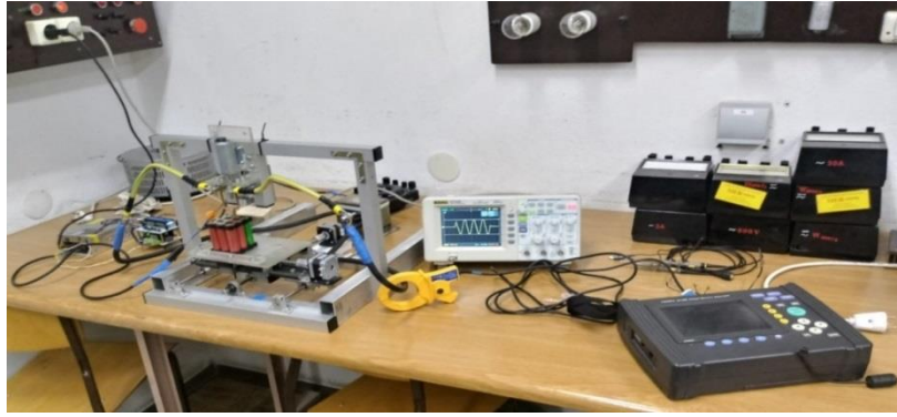
Figure 1 – Automatic spot welder device (at the left) on the measuring stand
