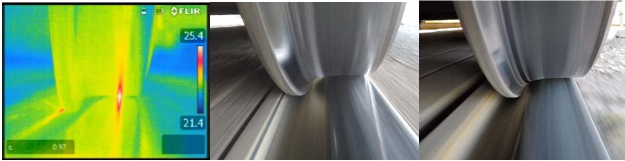
Fig. 2. Thermal and visible light images of wheel-rail interface
